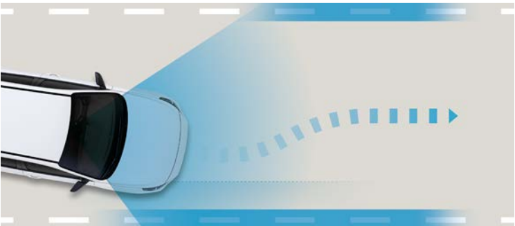
Lane Keeping Assist (LKA). At speeds over 60 km/h the system alerts the driver about unsafe movements. In case of an unintended lane departure, it will warn the driver and can apply counter steering torque to guide the car back to a safe position.
