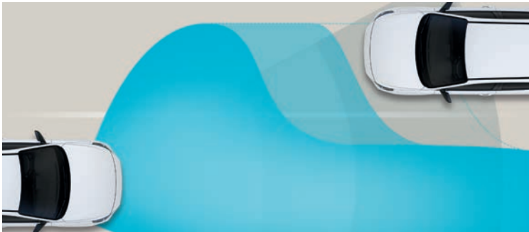
High Beam Assist (HBA). High Beam Assist detects oncoming vehicles as well as vehicles in the same lane ahead at night, and automatically changes from high beam to low beam as appropriate.
