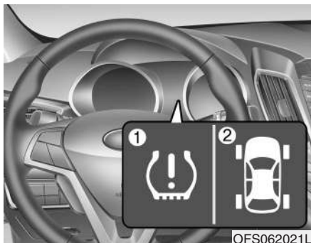
(1) Low tire pressure telltale / TPMS malfunction indicator
