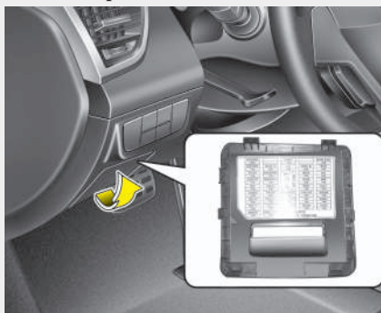
Inner fuse panel
